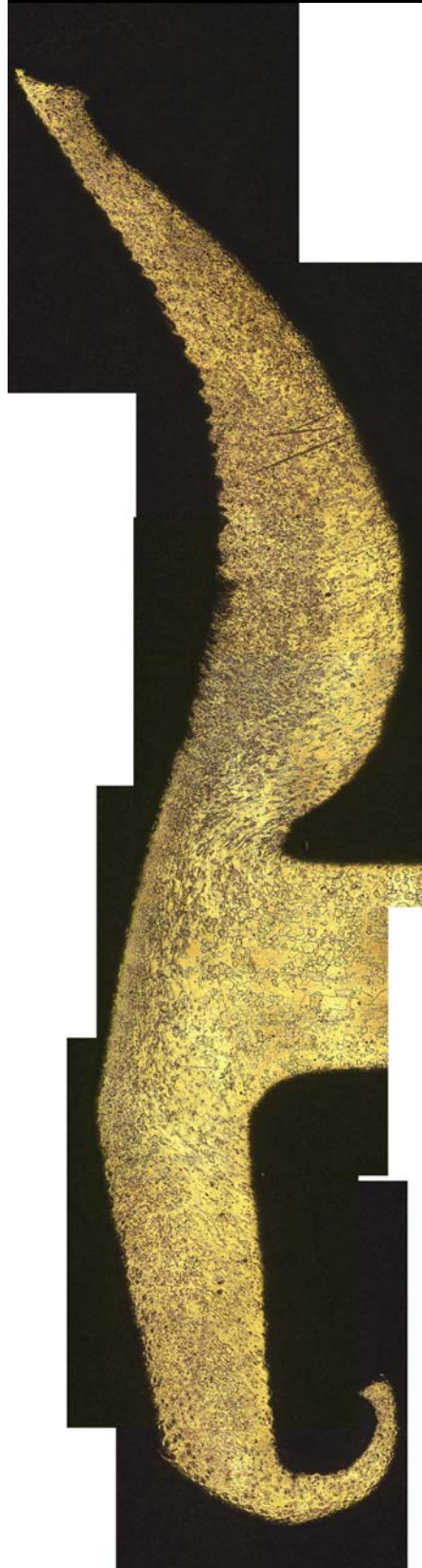
Photomicrographs – Flowdrilled Hole “A”
