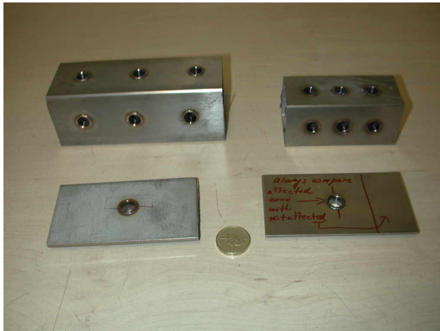
Fig 1. General photograph showing the range of Flowdrilled samples submitted for Examination
